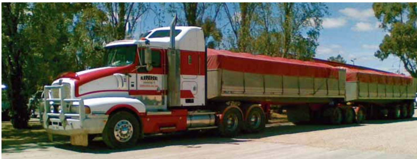
The T604 Kenworth Prime Mover B-Double Combination that was repowered with a C15
