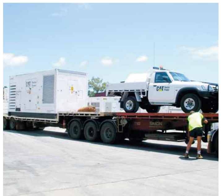
The 44 kVA Olympian GEP 44-5 generator set installed on the Thiess concept service vehicle.
