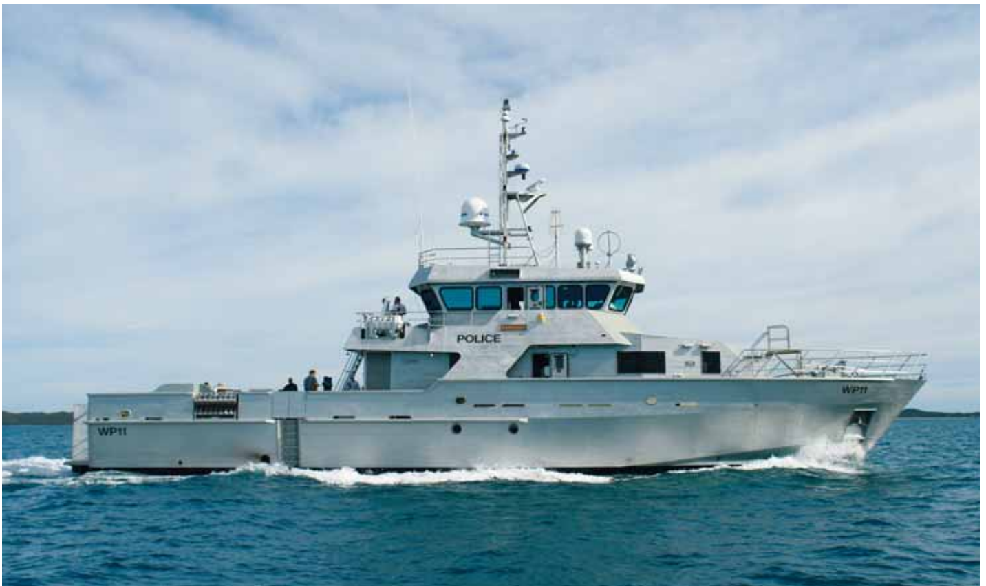
The C32's exceptional torque output gets the 'Nemesis' out of the water fast and produces sprint speeds of 27 knots.
