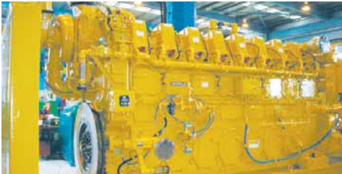
The centre's first Caterpillar G3608 Gas Engine rebuild was recently undertaken for Santos.
