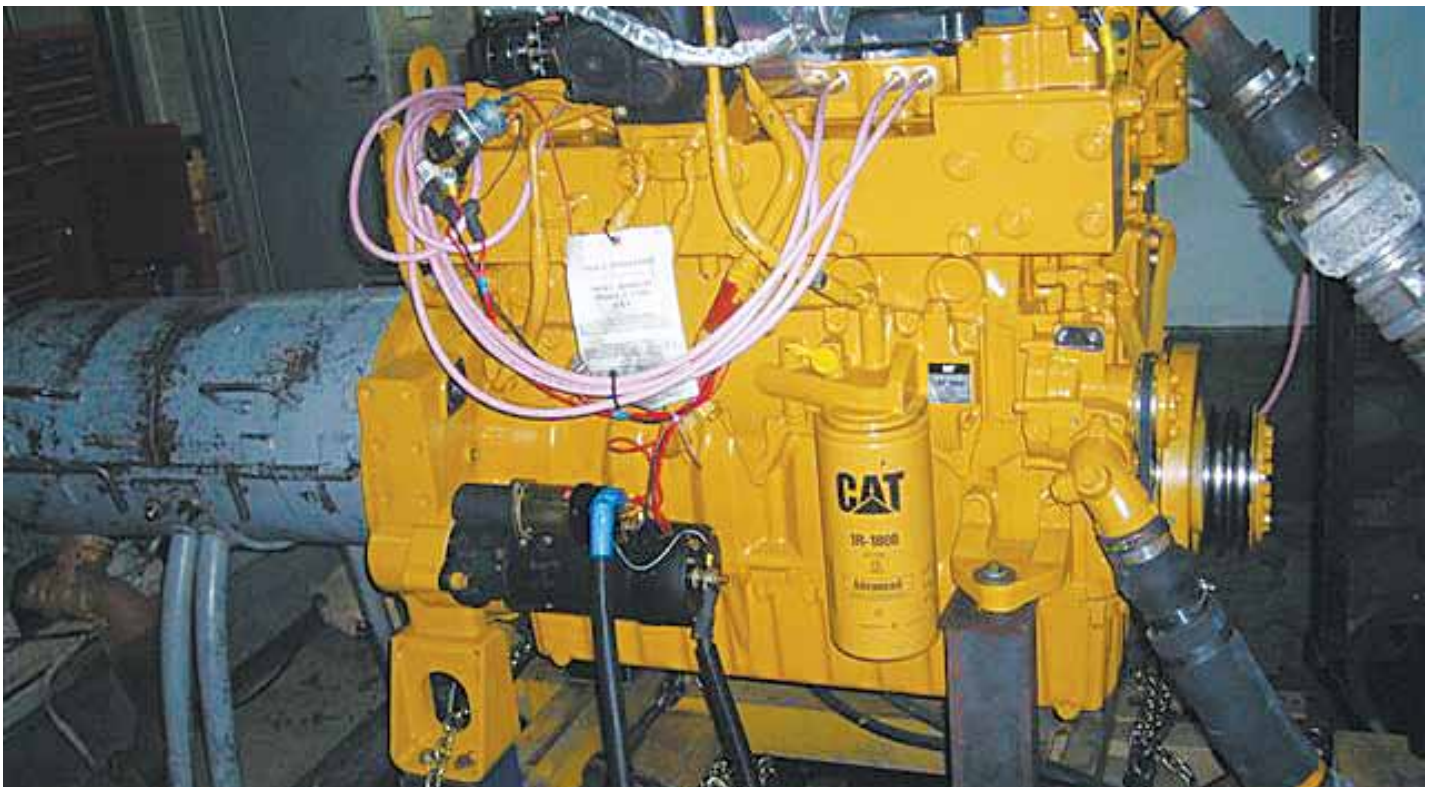
A C9 engine being put through its paces at the WesTrac dyno facility.
