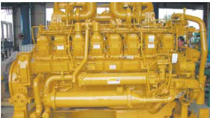
A Parts Exchange Caterpillar 3516 engine from a 793 truck.
