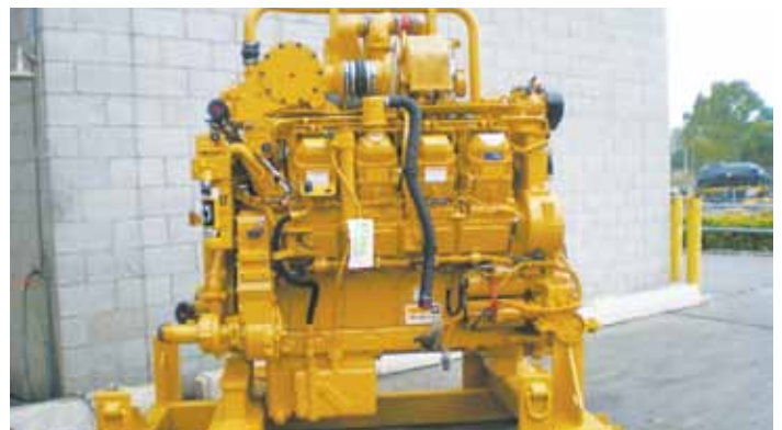
A Parts Exchange Caterpillar 3508 Engine from a D11.
