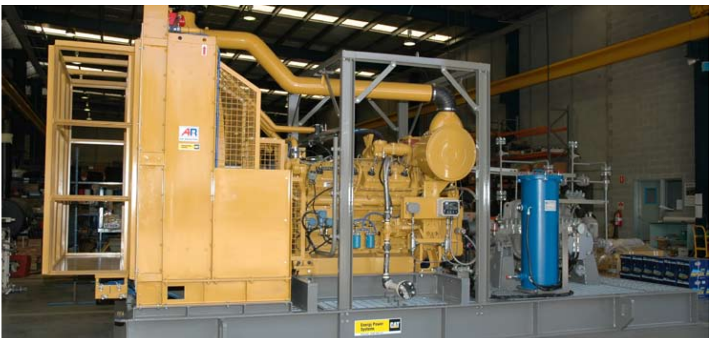
The gas engine-driven G3412 Pumping Package is nearing completion.
