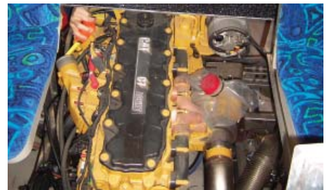
Bustech's midi engine hatch fitted with a Caterpillar C7 ACERT engine.
